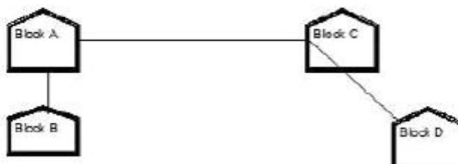
e2) The most suitable place / block to house the server of this organisation would be Block C, as this block contains the maximum number of computers, thus decreasing the cabling cost for most of the computers as well as increasing the efficiency of the maximum computers in the network.
