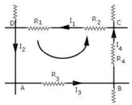
This gives:  $(R_1 + R_2) I_1 + R_3 I_3 + R_4 I_4 = 0$
