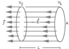
the material through which a current is passing along the length, normal to the area A. But, JA = I, the current through the area A and  $EL = V_1 - V_2$ , the potential difference across the ends of the cylinder denoting  $V_1$ - $V_2$  as V,
